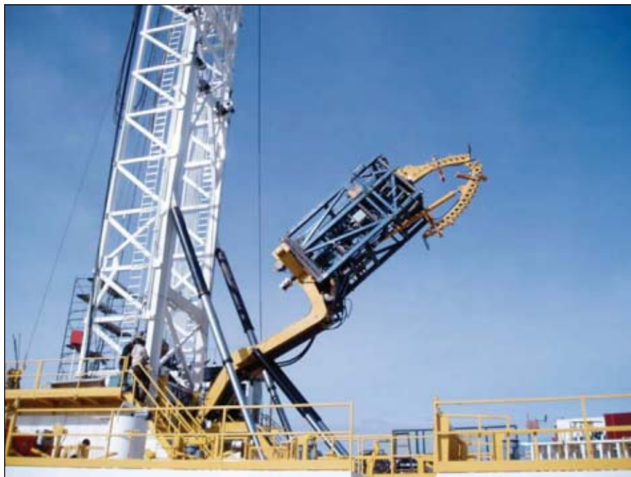
The top drive of the XTC 400 coil-over-top-drive rig can swing in and out of the derrick (Fig. 4; photo from Xtreme Coil Drilling Corp.).
